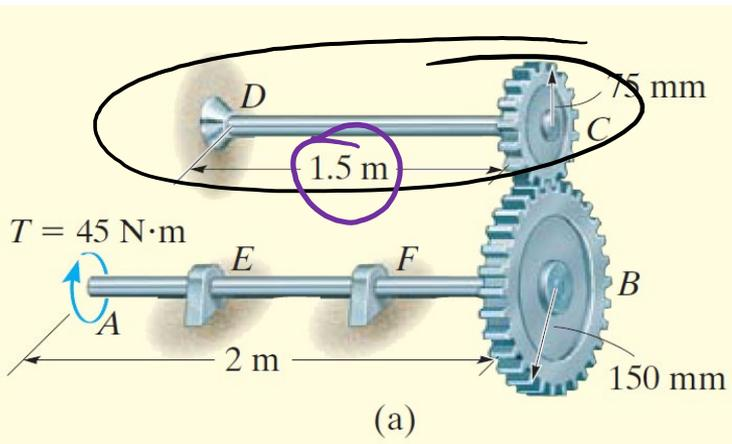
Two solid steel shafts are connected through gears at points B and C. The top shaft is mounted to a fixed wall at point D. Determine the angle of twist at point A assuming a torque of  $T = 45 \text{ N}\cdot\text{m}$  is applied at A. Each shaft has a diameter of  $d = 20 \text{ mm}$  and a shear modulus of  $G = 80 \text{ GPa}$
