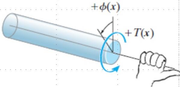
Just as the torque follows the right-hand rule, so does the twist  $\phi$ .
