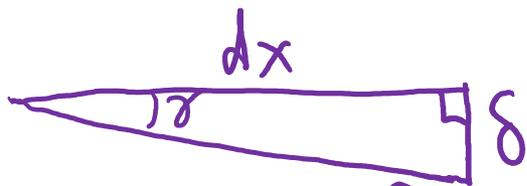
$$\tan \gamma = \frac{\delta}{dx} = \frac{\rho \cdot d\phi}{dx} = \rho \cdot \frac{d\phi}{dx}$$
