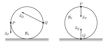
Which body does *not* have physically possible accelerations for points P and Q?
