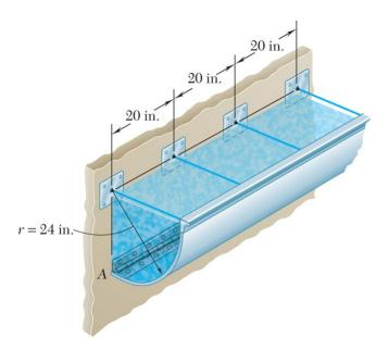
b) Calculate the horizontal component of the equivalent hydrostatic pressure force on the trough, and the corresponding  $\bar{y}$  location measured from A.
