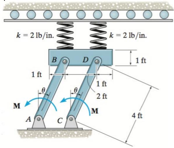
Determine the angel of equilibrium,  $\theta$ , given that block D has a mass of 7 kg and the links each have a mass of 3 kg.
