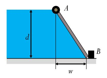
Determine the magnitude of the support reaction at the gate stopper B. The water level is d = 4 m, w = 3 m, and gate AB has a width of 2 m.
