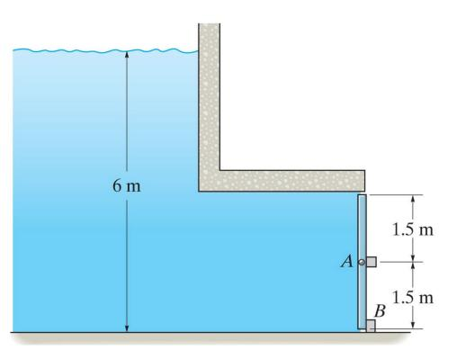
The 2-m-wide rectangular gate is pinned at its center A and is prevented from rotating by the block at B. Determine the reactions at these supports due to hydrostatic pressure.
