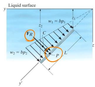
Determine the magnitude of the resultant force acting on the 100-m wide dam due to hydrostatic pressure. Let  $d=2.5~\mathrm{m}$ .
