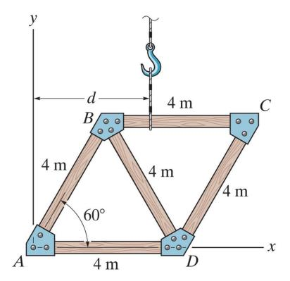
The truss is made from five members, each having a length of 4 m and a mass of 7 kg/m. Determine the distance *d* to where the hoisting cable must be attached, so that the truss does not tip (rotate) when it is lifted.
