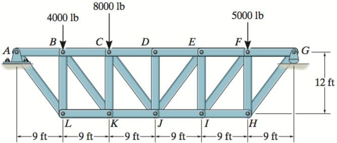
Determine the force in members *BF*, *BG*, and *AB*, and state if the members are in tension or compression.
