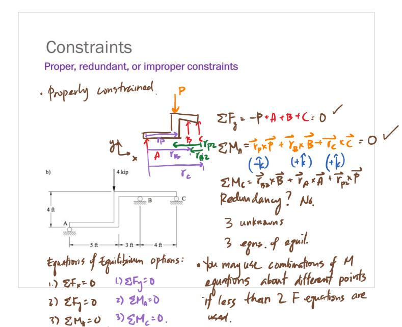
Proper, redundant, or improper constraints
