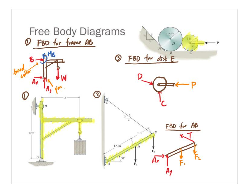
To ensure equilibrium of a rigid body, it is not only necessary to satisfy equations of equilibrium, but the body must also be properly constrained by its supports
