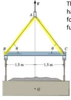
The lift sling is used to hoist a container having a mass of 500 kg. Determine the force in each of the cables AB and AC as a function of  $\theta$ .
