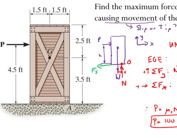
Find the maximum force P that can be applied without causing movement of the crate. Given:  $\mu_s = 0.4$ , W=250lb
