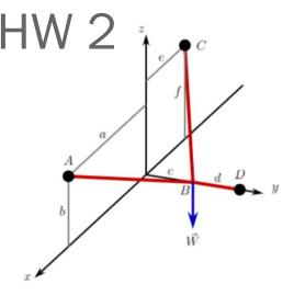
Write out system of equations based on the FBD @ point B
