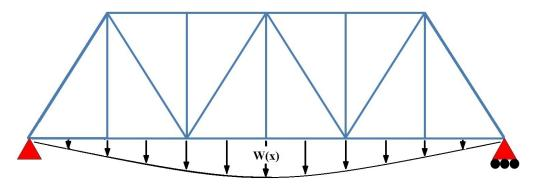
f) The above truss has the same dimesions as the previous with a distributed load given by  $W(x) = \frac{100x}{a} \left(\frac{x}{a} - 6\right)$ . Obtain expressions for the external forces at A&G as a function of a. Analyze how the distributed load change the system.
