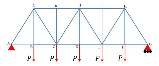
a) Draw a free body diagram of the truss and obtain expressions for the external reaction forces at A and G as a function of P and a.
