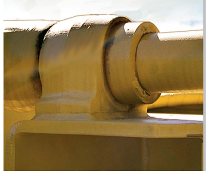
This thrust bearing is used to support the drive shaft on a machine. (7)
