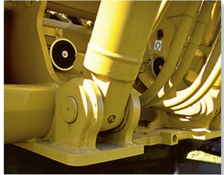
This pin is used to support the end of the strut used on a tractor. (8)
