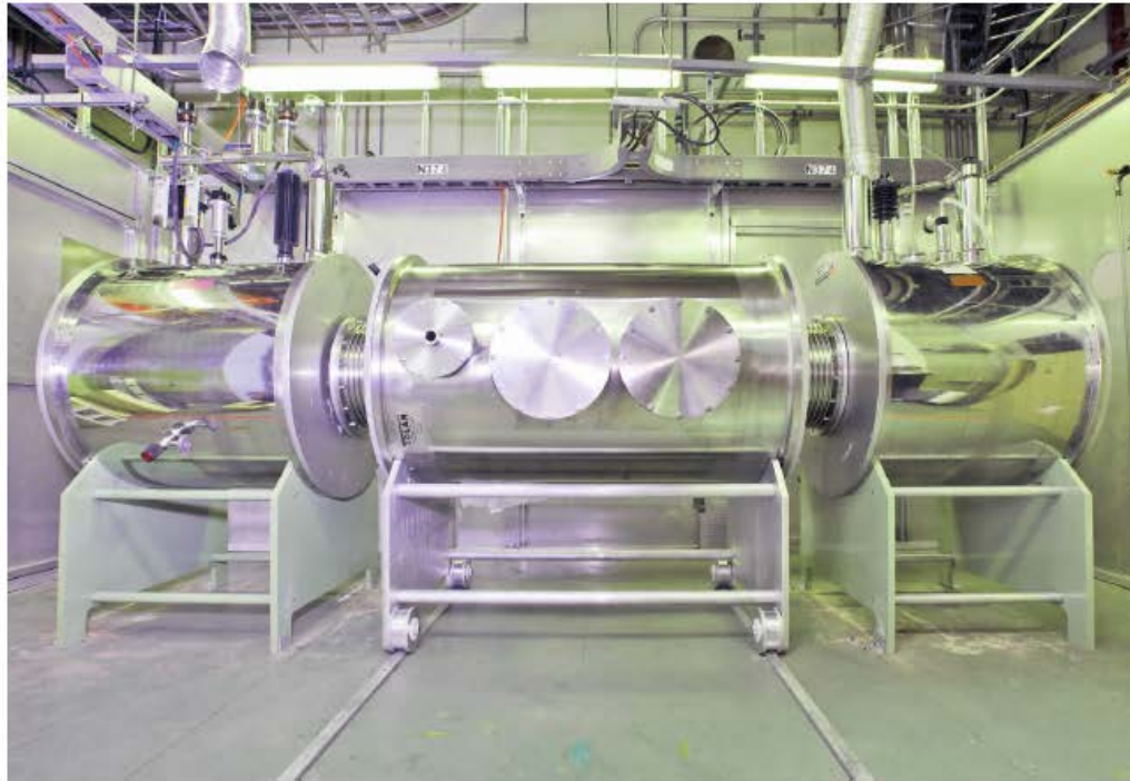
Figure 2: The small-scale PTOLEMY prototype installed at the Princeton Plasma Physics Laboratory (February 2013). Two horizontal bore NMR magnets are positioned on either side of a MAC-E filter vacuum tank. The tritium target plate is placed in the left magnet in a 3.35T field, and the RF tracking system is placed in a high uniformity 1.9T field in the bore of the right magnet with a windowless APD detector and in-vacuum readout electronics.
