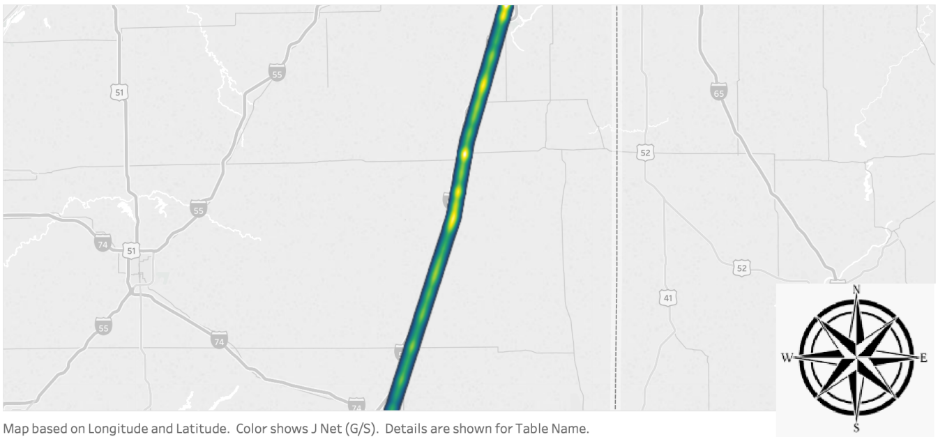
Figure 11: Magnified plot (vs. latitude) and jolt-density map of jerk measured on Chicago-Champaign Amtrak route. This magnified region was selected as it corresponds to a rough segment of track between Gilman and Kankakee, Illinois.
