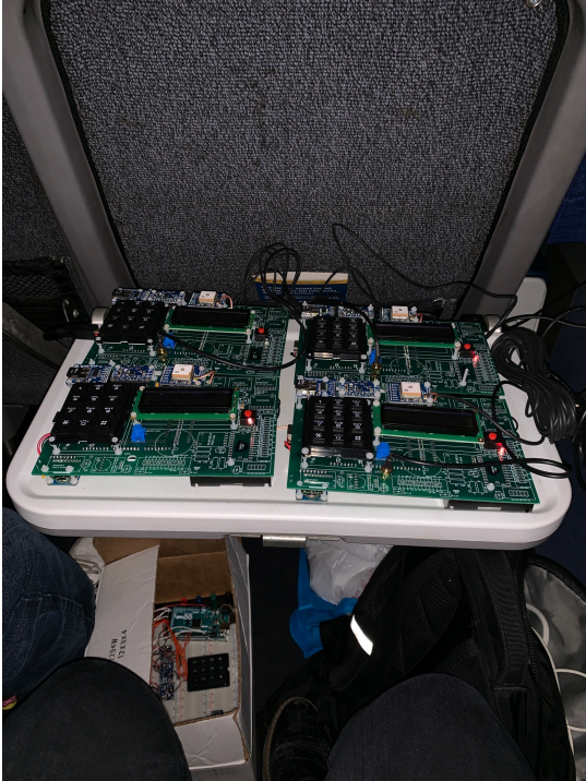
Four DAQ devices aboard an Amtrak train.
