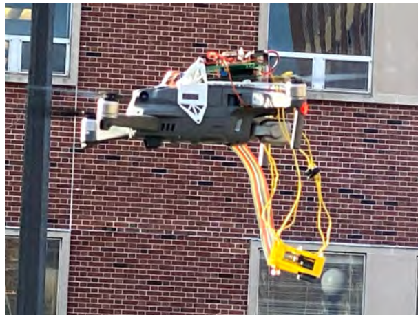
Image 2: Sensors and processor 3-D Printed Apparatus on Drone
