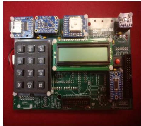
Figure 3: MicroSD, keypad, accelerometer, LCD, GPS, multiplexer, and BME 680 on the front of the PCB
