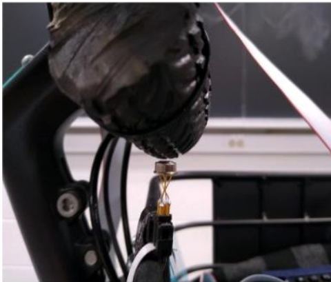
Figure 8: The infrared sensor pointed towards the control tire
