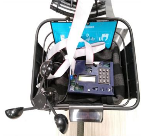
Figure 9: Printed circuit board and wind anemometer in the basket of the bike.
