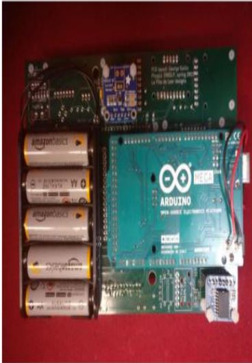
Figure 4: Battery pack, Arduino, and RTC mounted on the PCB
