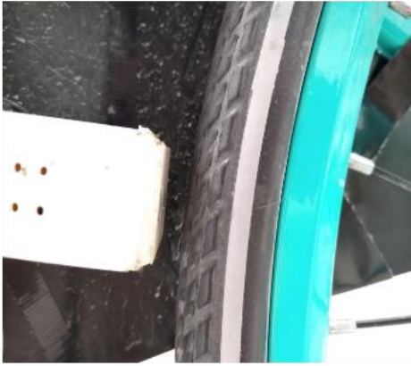
Figure 6: The two infrared sensors pointed towards the back tire of the Veoride
