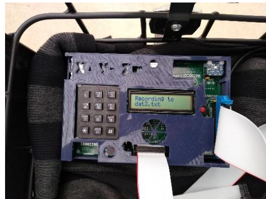
Figure 11: Printed circuit board recording data
