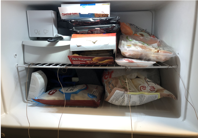
Figure 7: Freezer and thermocouples.
