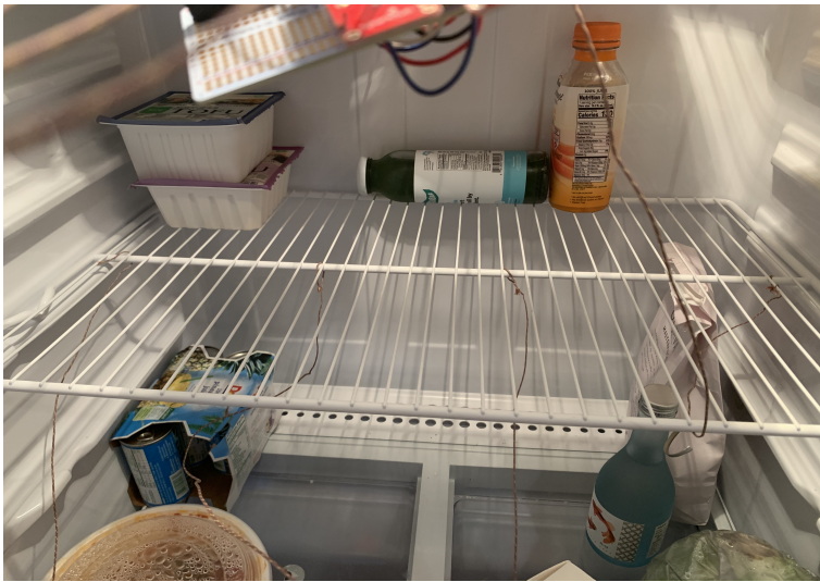
Figure 6: Fridge and thermocouples.
