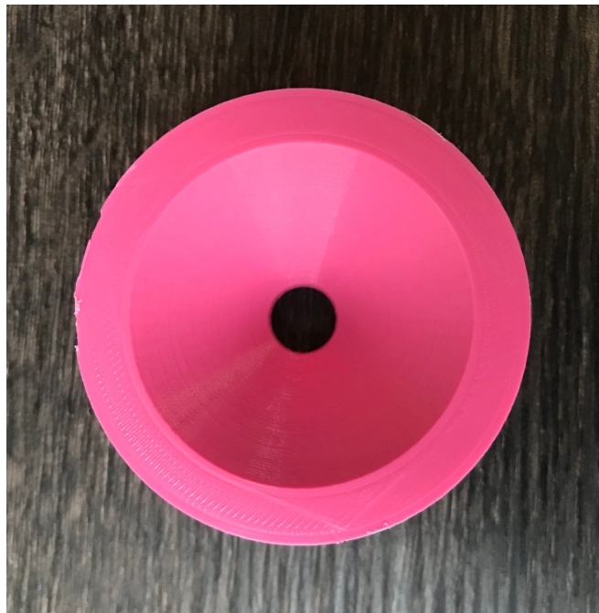
Figure 8: Top view of a 3-D printed stethoscope bell used in the data collection process
