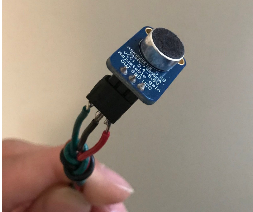
Figure 7: One of the two microphones attached to the printed circuit board using wires
