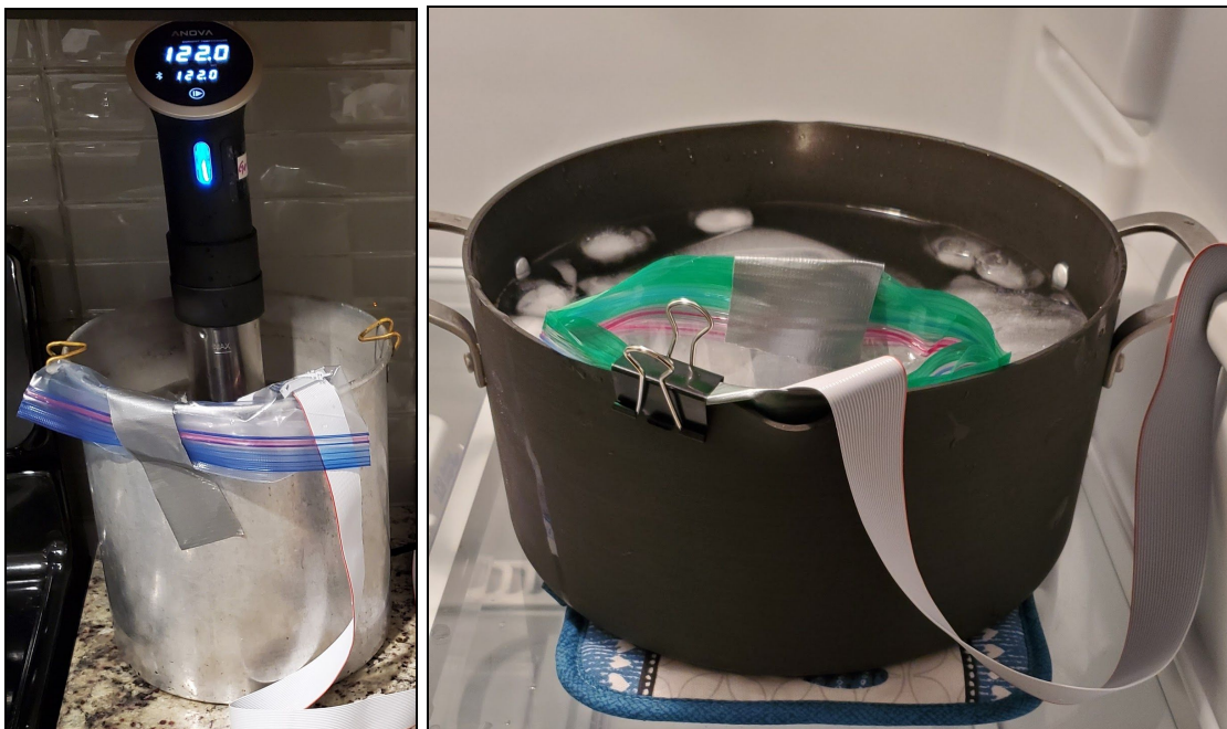
Figure 9: Measurements being taken in hot environment (left) using a sous vide to maintain constant 50°C temperature and cold environment (right) using a bath of ice water stored in the fridge to maintain constant 0°C temperature
