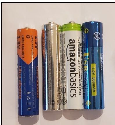
Figure 1: The batteries listed from left to right: 1.5V alkaline AAA, 1.5V lithium AAA, 1.2V nickel-metal hydride, 1.5V AAA lithium ion. Each will be tested under the variable conditions (discharge current & temperature)
