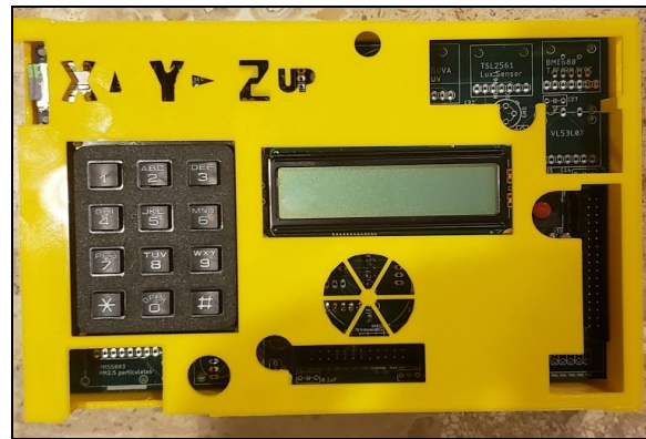
Figure 6a: Main DAQ Instrument (with 3D printed cover)
