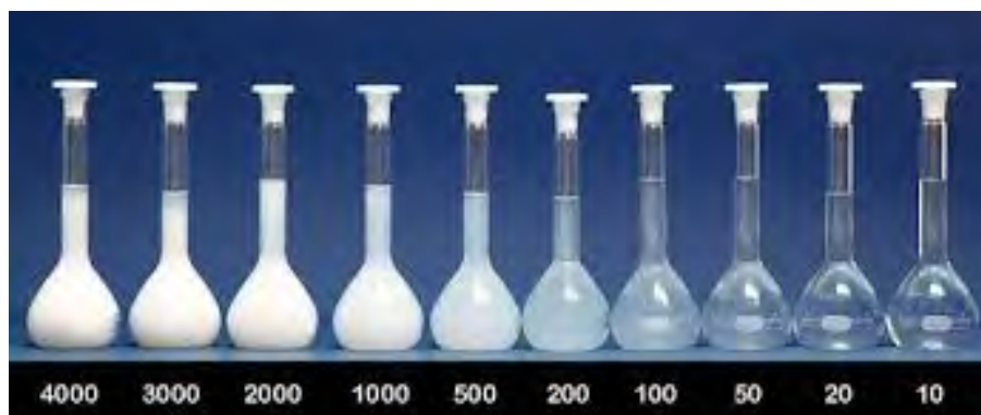
Figure 2.6: Representation of change in NTU and light transmittance
