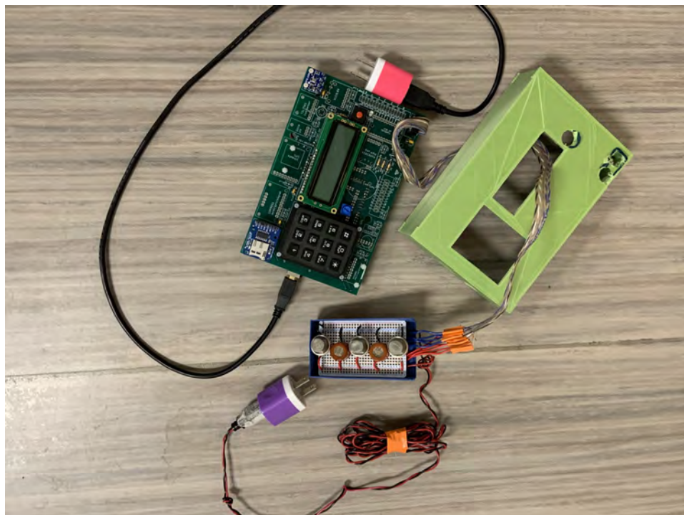
Figure 11: This shows our whole device. The Arduino and the heating elements of the sensors are powered by separately. The sensors are connected to the Arduino and rest of the components by a ribbon cable, which allows greater mobility for the sensors.
