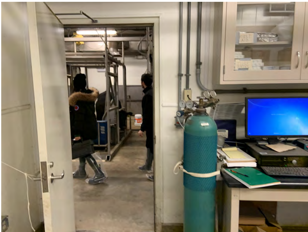
Figure 16: A door from the control room is open to the room with the stalls so some methane could also travel to the control room. However, we have compared the barn control sample with the calibration sample set-up in the lab away from the steers for added clarity.
