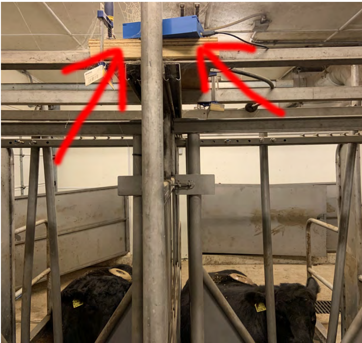
Figure 12: The red arrows point to one of our devices, placed on the wooden block directly over the steers. Another device is directly behind the blue device shown on the picture. A second device is set up at the same wooden block and can be seen in Figure 13
