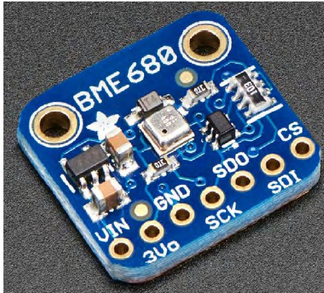
Figure 3: BME680. We used the I 2 C Clock and Serial Data In (SDI) pins visible in the image to connect to the SCL and SDA I 2 C lines, respectively. Figure adapted from Adafruit (2019).
