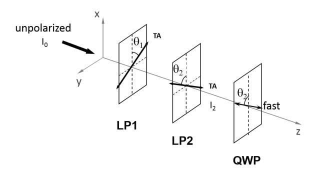
Unpolarized light of intensity  $I_0$  is incident on a linear polarizer (LP1) with transmission axis oriented at an angle  $\theta_1$ =15° clockwise with respect to the *x* axis. The light then passes through a second linear polarizer (LP2) with transmission axis oriented at an angle  $\theta_2 = 40^\circ$  counterclockwise relative to the *x* axis as shown before passing through a quarter wave plate. The fast axis of the quarter wave plate is also at an angle  $\theta_2 = 40^\circ$ .
