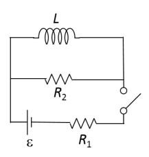
1) What is the voltage across the inductor just after the switch is closed?
