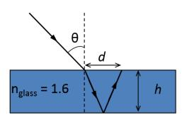
11) What is the distance d between where the incident ray enters and the reflected ray exits?
