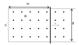
17) What is the current through the resistor when the metallic bar is a distance w = 0.225 m from the end sliding with a constant speed v = 4 m/s?
