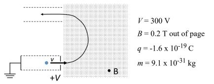
14) When the electron is in the magnetic field region, its speed v:
