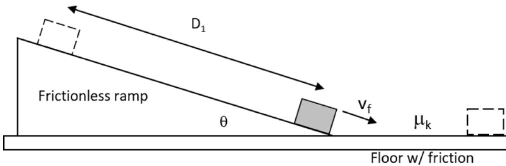
A 8 kg block starts at rest and slides down a frictionless ramp that makes an angle  $\theta=26$  degrees with respect to the horizontal floor below. At the bottom of the ramp, after having slid a distance  $D_1$ , the speed of the block is observed to be 12 m/s.
