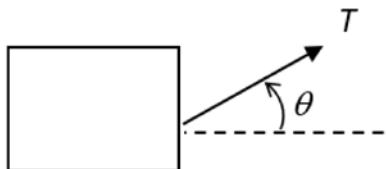
A physics student is trying to pull a box of books of mass  $m = 45 \text{ kg}$  across the floor as shown in the figure. The coefficient of static friction  $\mu_s = 0.42$  and the coefficient of kinetic friction  $\mu_k = 0.3$ .
