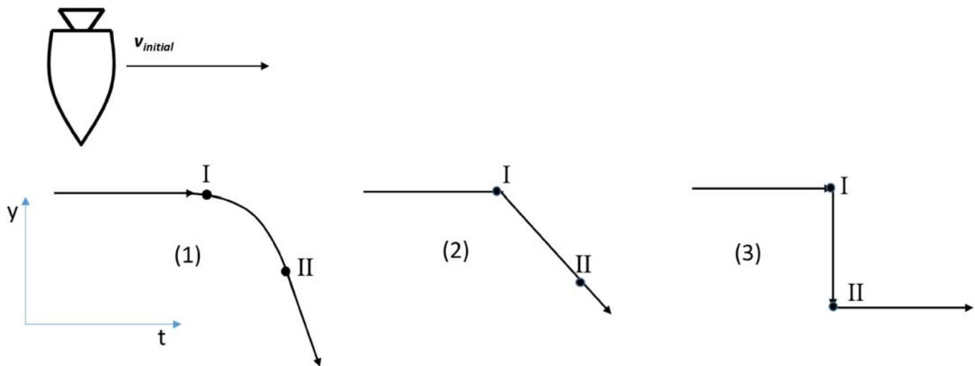
A rocket is drifting in deep space where gravitational forces are negligible. The rocket is initially drifting sideways ( $x$  direction) with its engine off as shown above. The engine, which generates a constant force in the  $-y$  direction, is then turned on (corresponding to point **I**) for 4 seconds, and then turned off again (point **II**).
