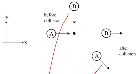
Two dry ice pucks slide on a horizontal, frictionless surface. Puck A, which is 2 kg, moves at speed 7 m/s in the positive x direction and Puck B, which is 1 kg, moves at speed 8 m/s in the negative y direction as shown in the figure. The pucks collide near the star in the figure. After the collision Puck B is moving in the positive x direction, while Puck A is moving in the direction that makes 45 degrees with the positive x-axis as illustrated.
