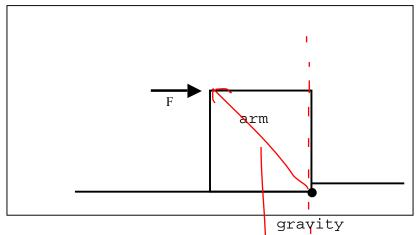
1. A solid, uniform cube 1 meter on a side is pushed against a narrow step on the floor (see figure); the block is then free to rotate about the axis marked with a solid black dot. A force F = 13N is applied horizontally to the edge opposite the narrow step. What is the magnitude of the torque around the axis marked by the black dot due to the force F?
