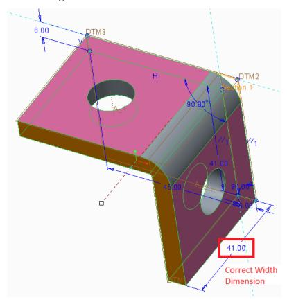
f. Regenerate the model and note the changes. (Hint: Select each hole and observe the dimensions - by selecting "Edit" - used to reference the hole positions.)
