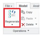
Your model may have already regenerated. In older versions of Creo, regeneration was not automatic. It is still good practice to regenerate the model after editing it. Regeneration rebuilds the model from scratch on the computer. For complex models, even though the model may appear regenerated, certain features may not have regenerated. Regeneration ensures that the model is displayed correctly.
