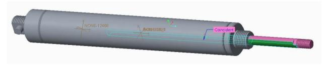
5) After selecting the rotation axes, go back to the "Placement" tab in the assembly ribbon. Notice that Creo now requests that we select "Rotation" constraints.
