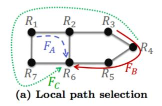
Centralized TE using SDNs allows closer to optimal routes.
