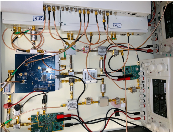
FMCW Baseband Circuit
