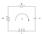
Use these laws to derive a dynamical model of this circuit which takes the form  $\dot{x} = A(t)\dot{x} + B(t)u$ .
