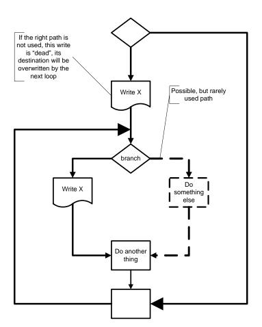
The compiler does not know that the right path is rarely used, so it cannot remove the first Write X instruction. The typical path, however, can be recorded from the ROB, stored and be used if the PC of the beginning of this trace is fetched again.
