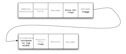
**Figure 1**: The new pipeline with the Store Set stage - changes in **bold**
