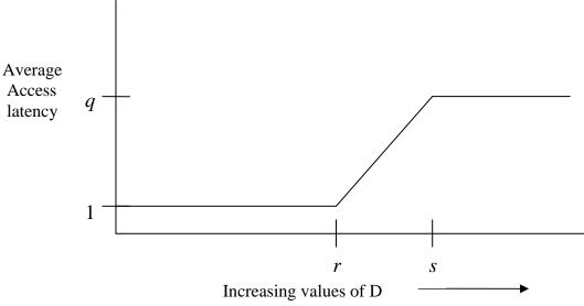
Using the values q, r, and s derived from this graph, along with p (L2 cache latency), determine the following properties of the L1 cache: (a) hit latency, (b) size, (c) line size, (d) associativity.
