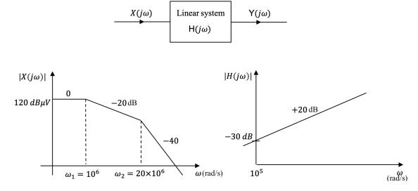
3. Determine the magnitude of the output of the system  $|Y(j\omega)|$  shown below at  $\omega = 50 \times 10^6$  rad/s.
