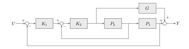
Compute the transfer function from the input U to the output Y.
