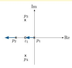
$$180^{\circ} = \angle L(s) = \angle \frac{s^m + b_1 s^{m-1} + \dots}{s^n + a_1 s^{n-1} + \dots}$$
