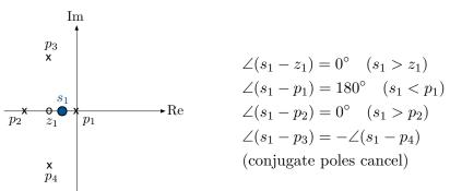
$$\angle(s_1 - z_1) - [\angle(s_1 - p_1) + \angle(s_1 - p_2) + \angle(s_1 - p_3) + \angle(s_1 - p_4)]$$
