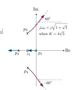
In Lab 5, you will need to select the value of gain K that corresponds to a desired pole on the root locus.
