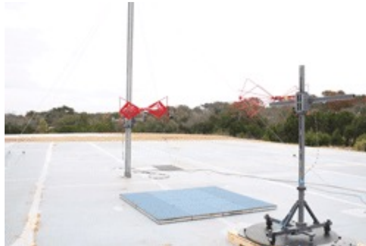
The outdoor set up for EMC measurement. Open Area Test Site (OATS)
