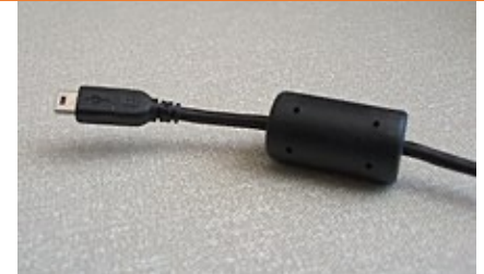
A ferrite bead at the end of a Mini USB cable
