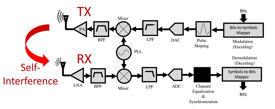
(1) Self-Interference saturates the Amplifiers & ADCs(2) Self-Interference results in negative SINR of RX signal
