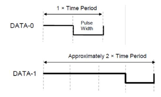
• Reader-to-Tag Encoding: Pulse Interval Encoding (PIE)
