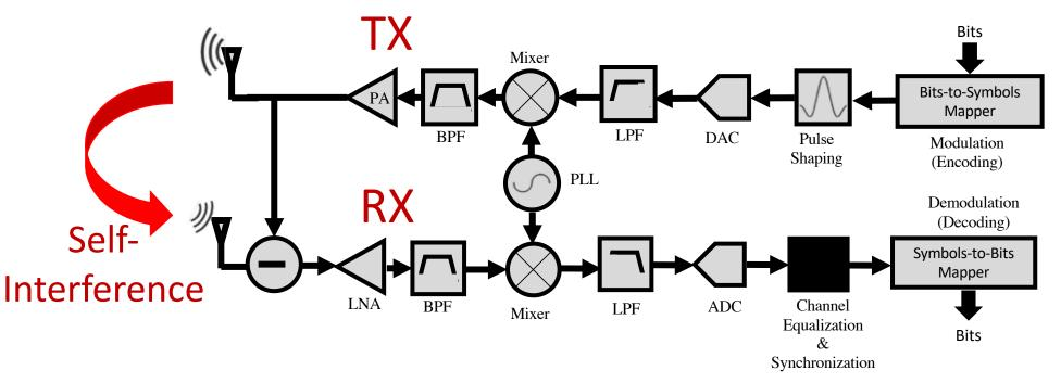
Self-Interference saturates the Amplifiers & ADCs
