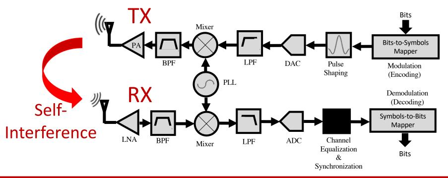
Self-Interference saturates the Amplifiers & ADCs
