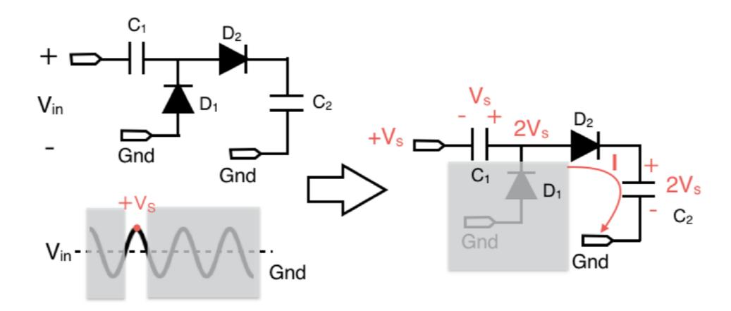
Multi-Stage Energy Harvesters can be used to amplify the voltage. (N stages  $\rightarrow$  NVs)
