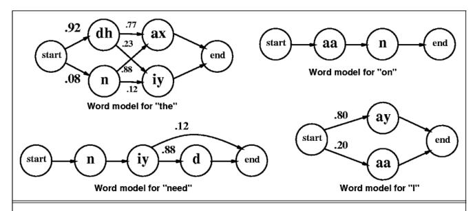
**Figure 7.5** Pronunciation networks for the words *I*, *on*, *need*, and *the*. All networks (especially *the*) are significantly simplified.
