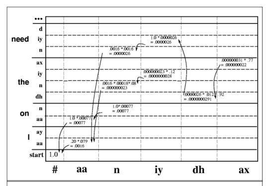
**Figure 7.10** The entries in the individual state columns for the Viterbi algorithm. Each cell keeps the probability of the best path so far and a pointer to the previous cell along that path. Backtracing from the successful last word (*the*), we can reconstruct the word sequence *I need the*.
