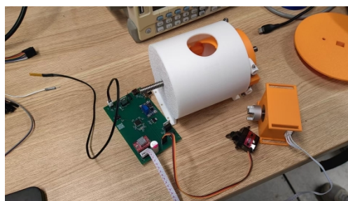
Figure 5. Integrated rotary extrusion and control assembly.
