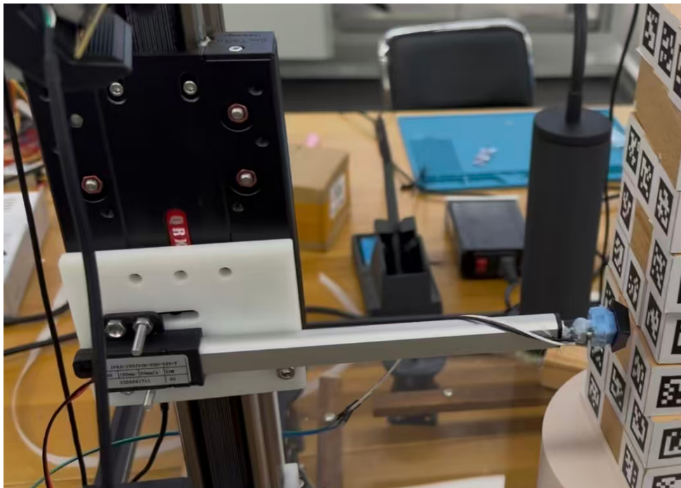
Figure 6: Pushrod unit of the JengaBot system.
