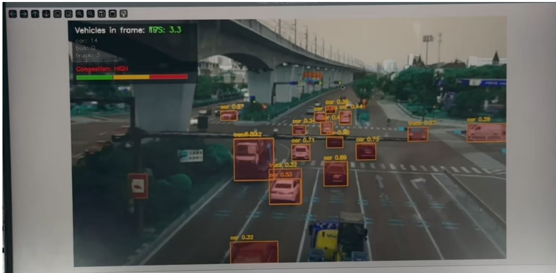
Figure 6: Vehicle detection output under high congestion.
