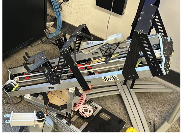
(b) Launcher and staging hardware.
