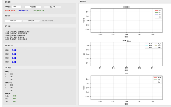
Figure 2.5: PC GUI for UDP reception, live signal visualization, and session saving.
