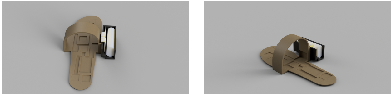
Figure 2.1: Mechanical insole CAD layout with side electronics container and routed sensor paths.
