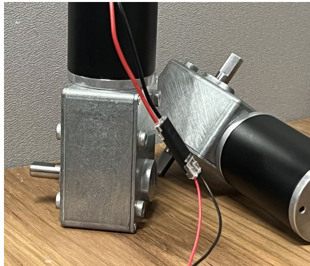
Figure 3: Motorized orientation mechanism for projector pre-alignment.
