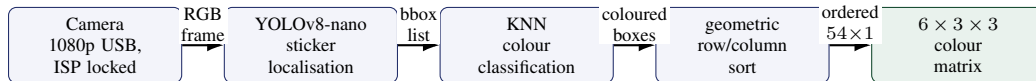
Figure 7: Decoupled vision pipeline. Locking the camera’s auto-exposure and white balance stabilises RGB values when the white 3D-printed arms enter the field of view; YOLOv8 then performs class-agnostic sticker detection, KNN assigns a colour to each bounding box, and a geometric sort emits the 6 \times 3 \times 3 matrix consumed by the Kociemba solver.
