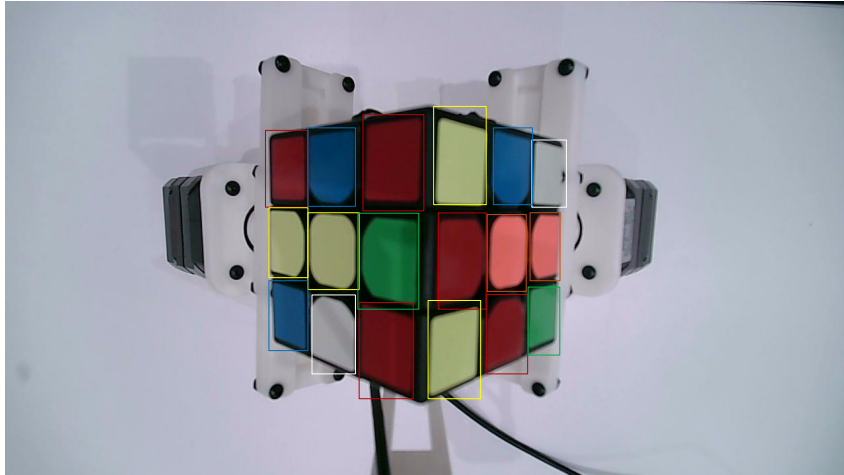
Figure 9: Integrated output of the vision pipeline on a representative frame: YOLOv8 has localised every visible sticker (bounding boxes), and KNN has assigned a colour class to each one (label colour). Partially occluded pieces are still classified correctly.
