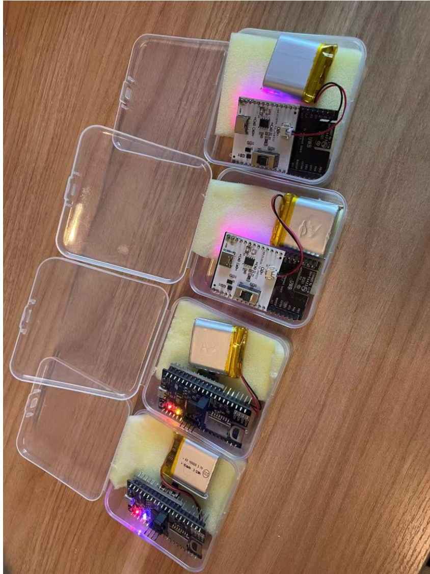
Figure C.1: Assembled UWB nodes and battery-powered prototype hardware.
