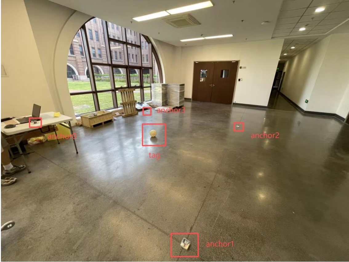
Figure 1.2: Indoor test field and UWB anchor layout used for prototype validation.
